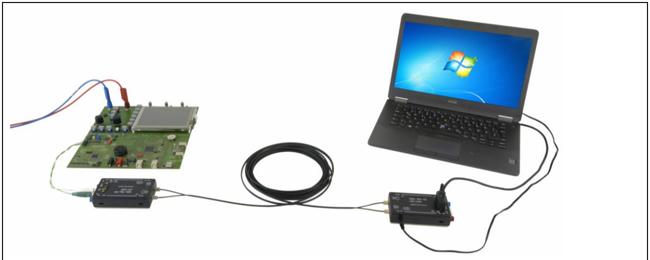
Figure 5: Two Opto-Boxes for data transmission connected via fiber optics
