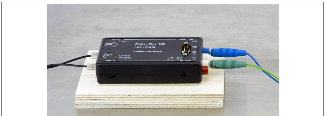
Figure 6: Opto-Box 100 operated isolated
